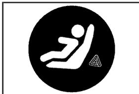
To assist you in locating the lower anchors for this child restraint system, each seating position with the LATCH system has a label on the seatback at each lower anchor position.
