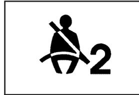
This chime and light will be repeated if the passenger remains unbuckled and the vehicle is in motion.
