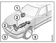
Engine-management system with catalytic converter
