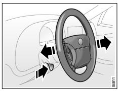
Lever for steering-wheel adjustment
