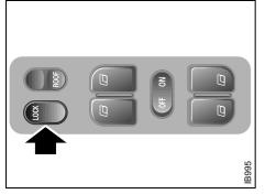
Switch for operation of central locking
