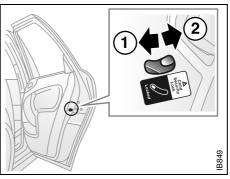
Child safety lock catch 1 Engaged 2 Disengaged
