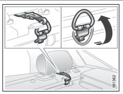
Child tether anchorage, Coupé and 5door models. The tether strap is not a part of the child tether anchorage.
