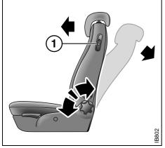
The backrest should be upright during driving, so that the safety belt, airbag and backrest can provide optimum protection in the event of emergency braking or a collision.
