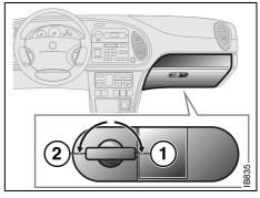
*Glove compartment* 1 To unlock 2 To lock
