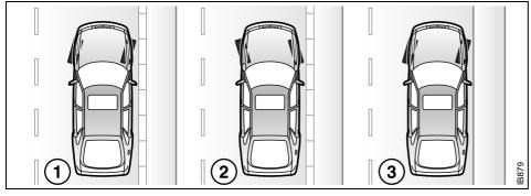
1 Pointing downhill and against the curb – Turn the wheels into the
