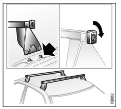
Mounting holes for load carrier, front on Coupés and front/rear on five-door models B883
