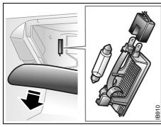
Glove-compartment lighting (detach the whole lamp unit with a short screwdriver applied at the lower edge)
