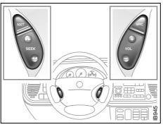
Audio System controls on steering wheel
