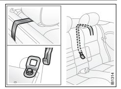
Attaching tether strap hook to anchorage, Convertible.
