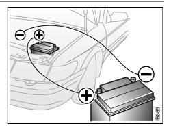
4 Open the hood and locate the battery. Find the positive (+) and negative (-) terminals on the battery.
