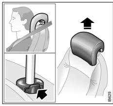
The head restraint can be raised or lowered and is adjustable in various positions.
