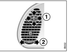
Dash vent 1 Adjusting the direction of the air flow. 2 Adjusting the air flow
