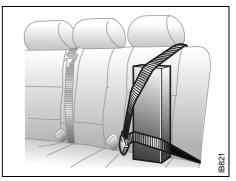
Securing a load on the rear seat
