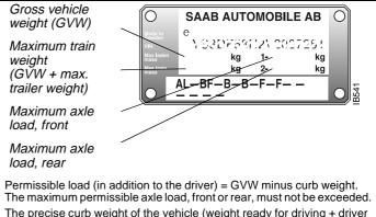
The precise curb weight of the vehicle (weight ready for driving + driver  $\acute{a}$  154 lbs. (70 kg) and load capacity are specified in the vehicle registration documents.
