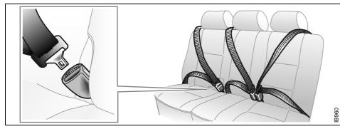
Safety belts, rear seat (the central head restraint is an accessory)
