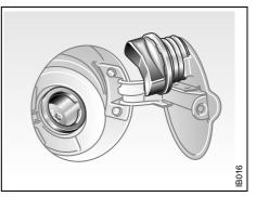
The most effective way to prevent condensation forming in the tank (and thus avoid possible running problems) is to keep the tank well filled.
