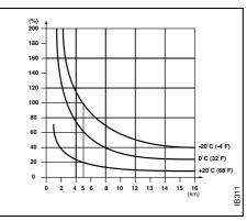
Percentage increase in fuel consumption of engine starting from cold compared to engine at normal temperature
