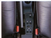
Switches for electric windows and switch to render door switches for rear windows inoperative
