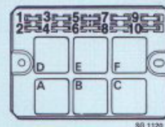
Power distribution panel on LH side, underneath rear seat
